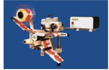
**Barcode reader** to control the barcode on the label, before it is applied. The reading result is compared with a master code, stored in the system memory and only if reading match this, the label is accepted.
